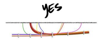
TIDY UP LOOSE OR STRAY WIRES AND HOSES IN THE COCKPIT.
