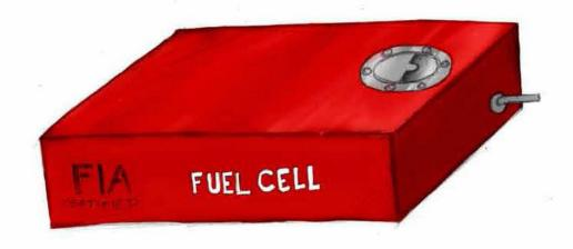
THE ONLY FUEL TANK THAT DOES NOT PEQUIPE A FULL METAL BULKHEAD BETWEEN IT AND THE DRIVER'S COMPARTMENT IS AN FIA CEPTIFIED FUEL CELL.
