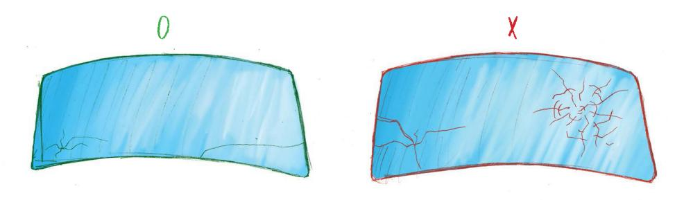
NO CRACKS OBSCUPING DRIVERS VISION. MINOR STARS AND CRACKS OUTSIDE OF DRIVERS VISION ARE DRAY, BUT NOTHING THAT CAN IMPEDE VISION OR COMPROMISE WINDSHIELD STRENGTH
